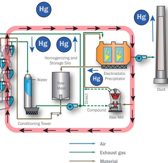
Hg cycle: Hg emissions are higher in direct operation than in compound operations.
