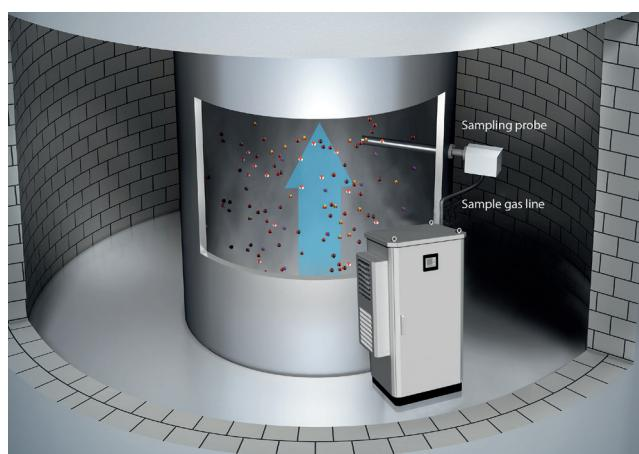
MERCEM300Z measures using hot extraction. The flue gas is extracted using a sampling probe and is transported to the analyser via a sample gas line. All components in contact with the sample gas, such as the probe, sample gas line, and converter in the analyser are heated above the dew point.
